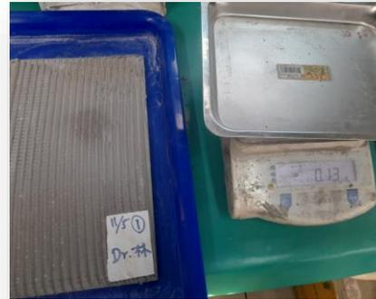
《 Anti-efflorescence test of tile adhesive 》
